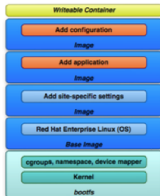
Figure 4: The layers of the Docker file system
